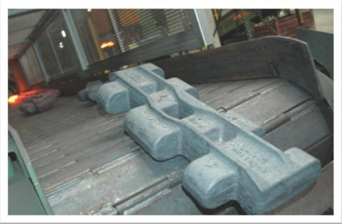
Controlled cooling system to ensure proper structure and surface of forgings.
