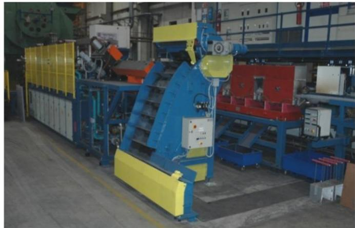
Double system of 3500 KW induction furnaces with temperature control.
