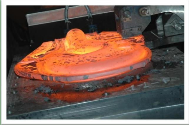
Electro-pneumatic die set up to manage even small batches and material change.
