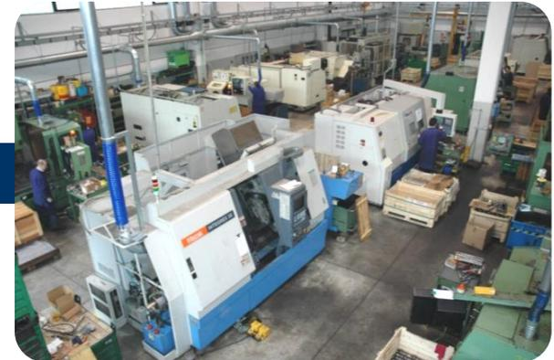
Forged parts became components ready to be used after machining operations
